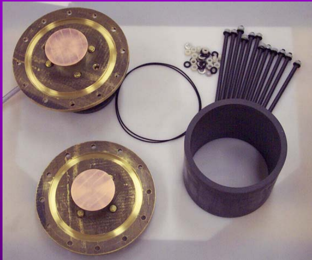
Aqueous high-power resistive load
