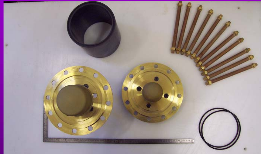
SF 6 pressurised spark-gap (components)
