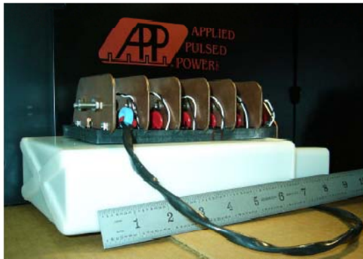
Fig 1. Solid state switch attached to a 0.15\mu\text{F} Capacitor
